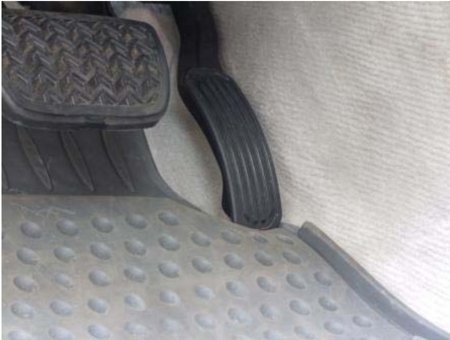
Example of an unsecured driver-side floor mat trapping the accelerator pedal in a 2007 Lexus ES350
