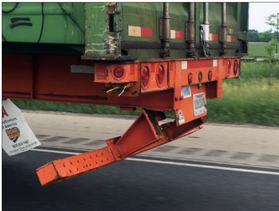
Figure 5: Example of a Damaged Rear Guard
