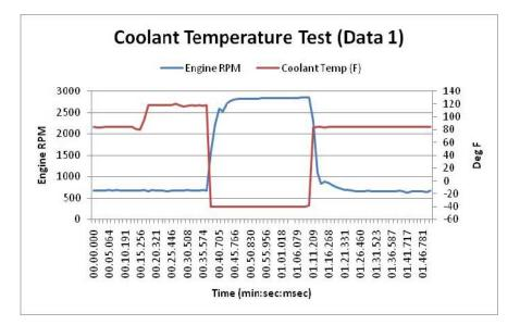
This engine temperature change would not happen in the real world. The NESC team mentions this, but later dismisses it. What would happen if this type of circuit fault were to occur with the vehicle in gear? *Significant torque output, unrequested by the driver, causing UA*.
