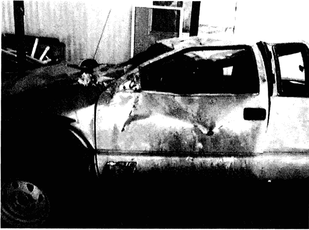
Figure 13. 1999-078-034, A-pillar Bending along its length (Driver Side View)
