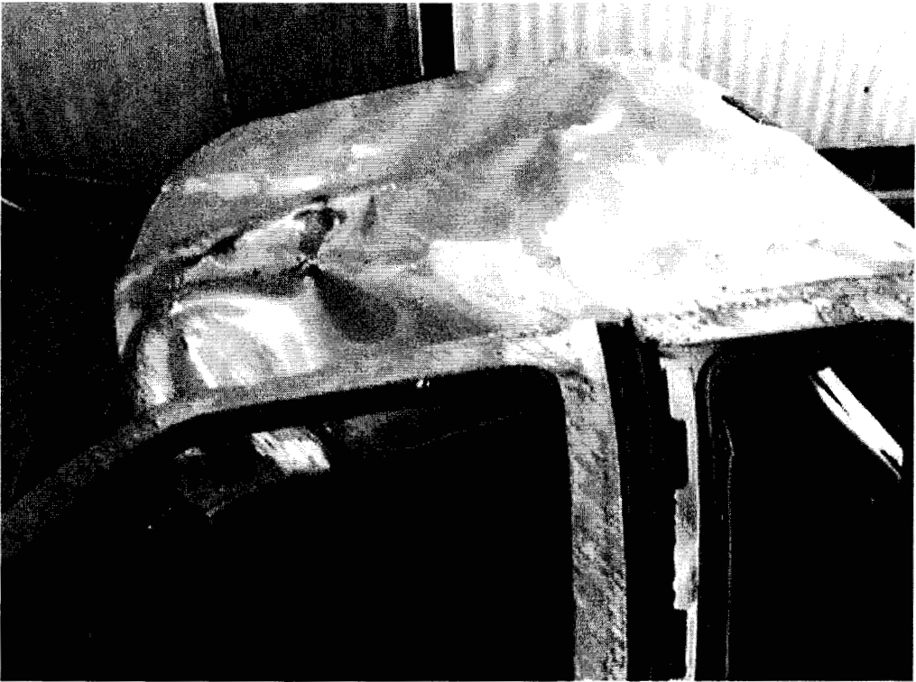
Figure 14. 1999-078-034, Roof Damage (Top View)
