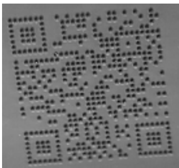
Figure 4. Example 2D barcode; QR code etched in rubber
