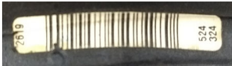
Figure 5. Example 1D barcode on tire bead
