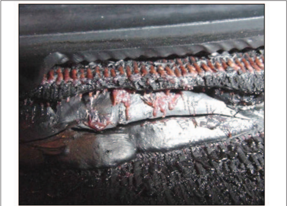
Figure 15.8: Melted polyester cord (lower sidewall)
