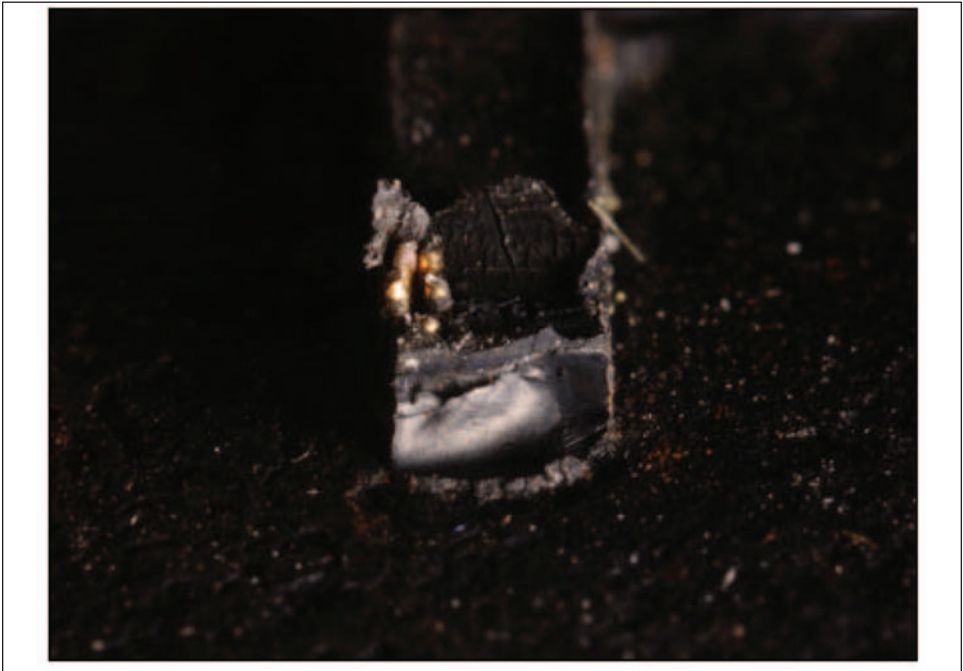
Figure 15.21: Steel cord tensile pull test, resulting in cord fracture
