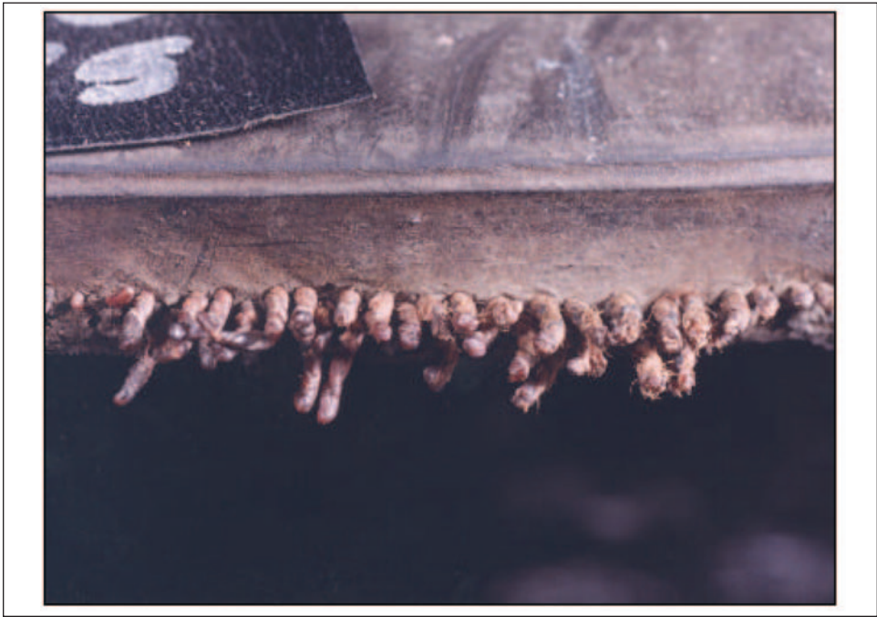
Figure 15.15: Broken, heat-fused polyester body cords, upper sidewall
