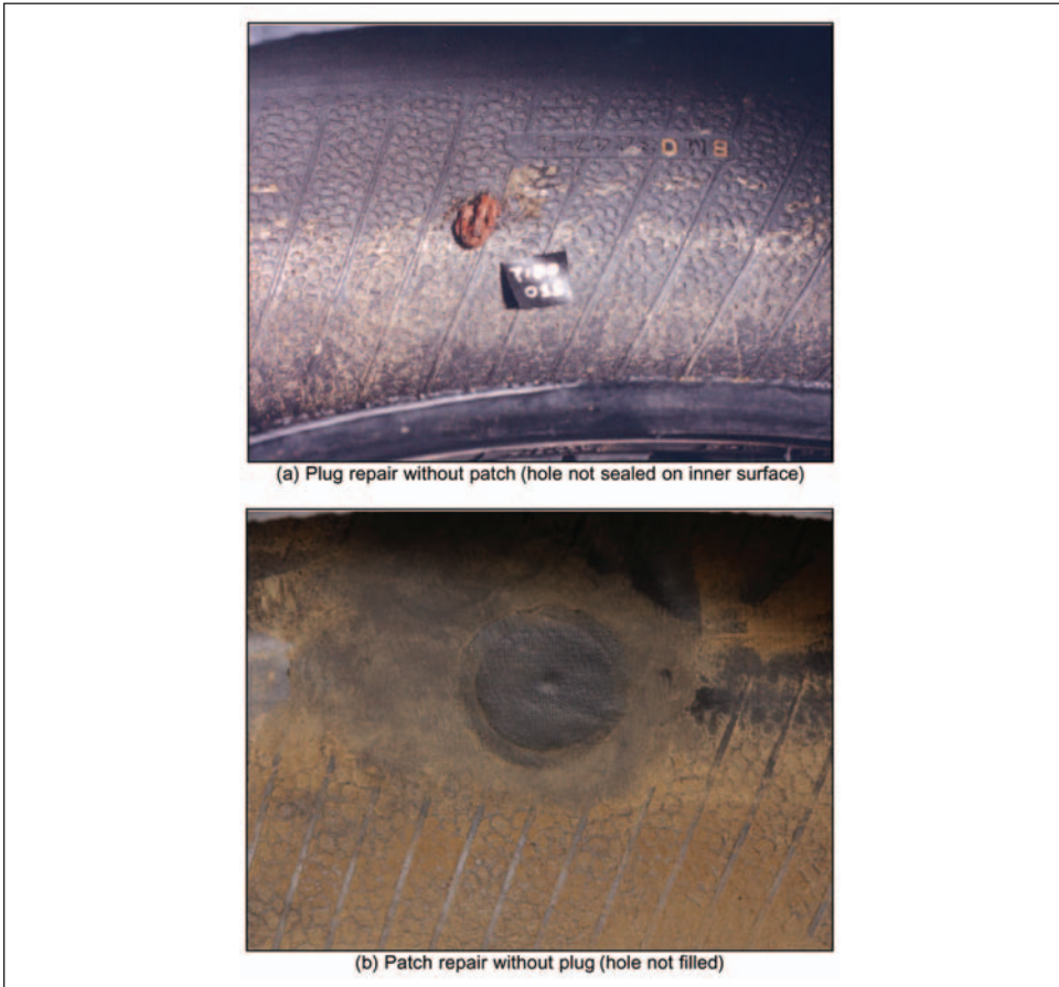
Figure 15.19: Examples of improper puncture repair
