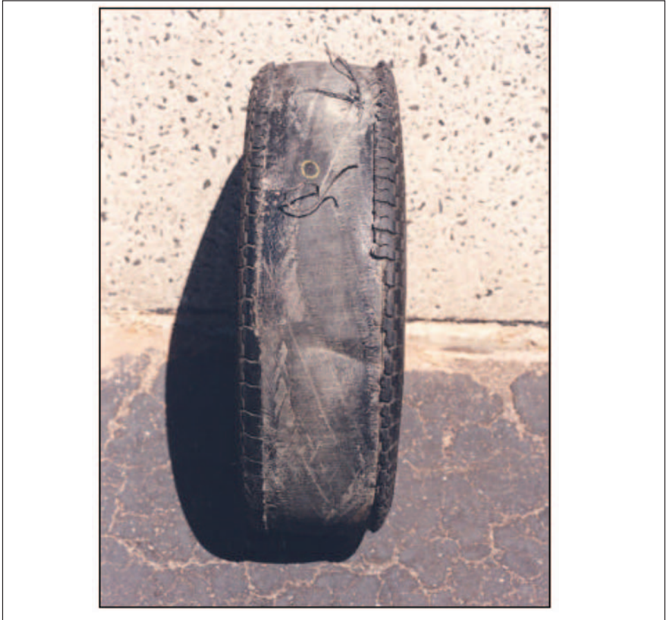
Figure 15.16: Exemplar tire after tread/belt detachment
