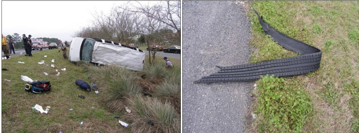
Figure 7. Lake City vehicle and tire; at left is a postcrash view of the 2002 Ford 15-passenger van at final rest on its left side, and, at right is the delaminated tire tread. (Source: Florida Highway Patrol)
