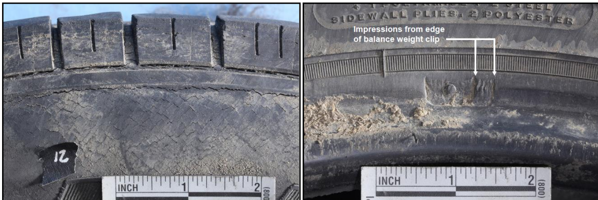
Figure 6. Centerville SUV tire; at left is the inboard sidewall exhibiting cracking on the sidewall, buttress, and shoulder; at right are the impressions left by the wheel weight clip near the bead on the inboard side of the tire.
