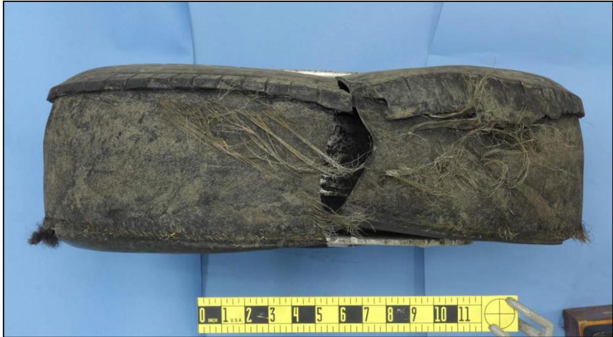
Figure 4. Detreaded tire carcass from the Centerville SUV.
