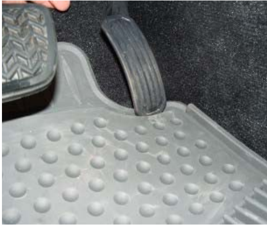
Example of accelerator pedal interference caused by out-of-position all-weather floor mat.
