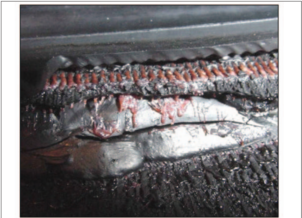
Figure 15.8: Melted polyester cord (lower sidewall)
