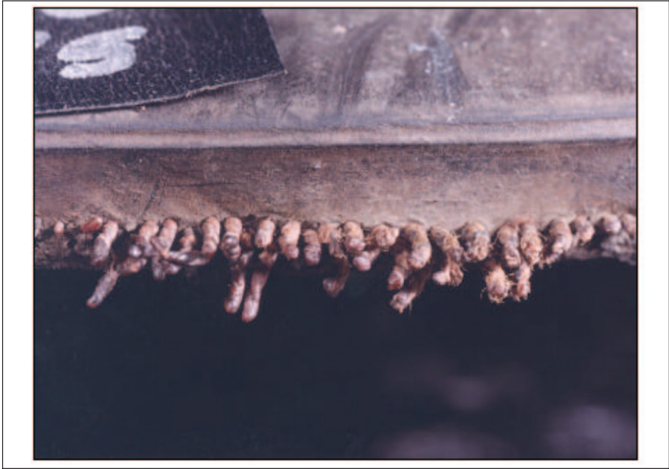
Figure 15.15: Broken, heat-fused polyester body cords, upper sidewall
