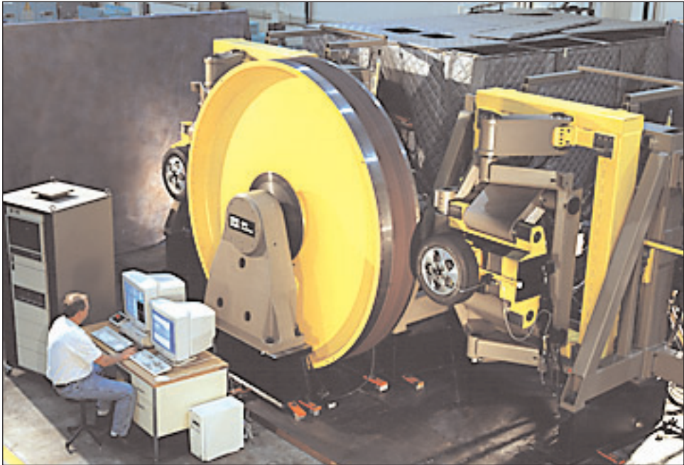
Figure 7.17: Relationship of tire, machine bed, and transducers during operation (reprinted from Tire Science and Technology, Vol. 27, No. 3, 1999 with Tire Society permission) [7]
