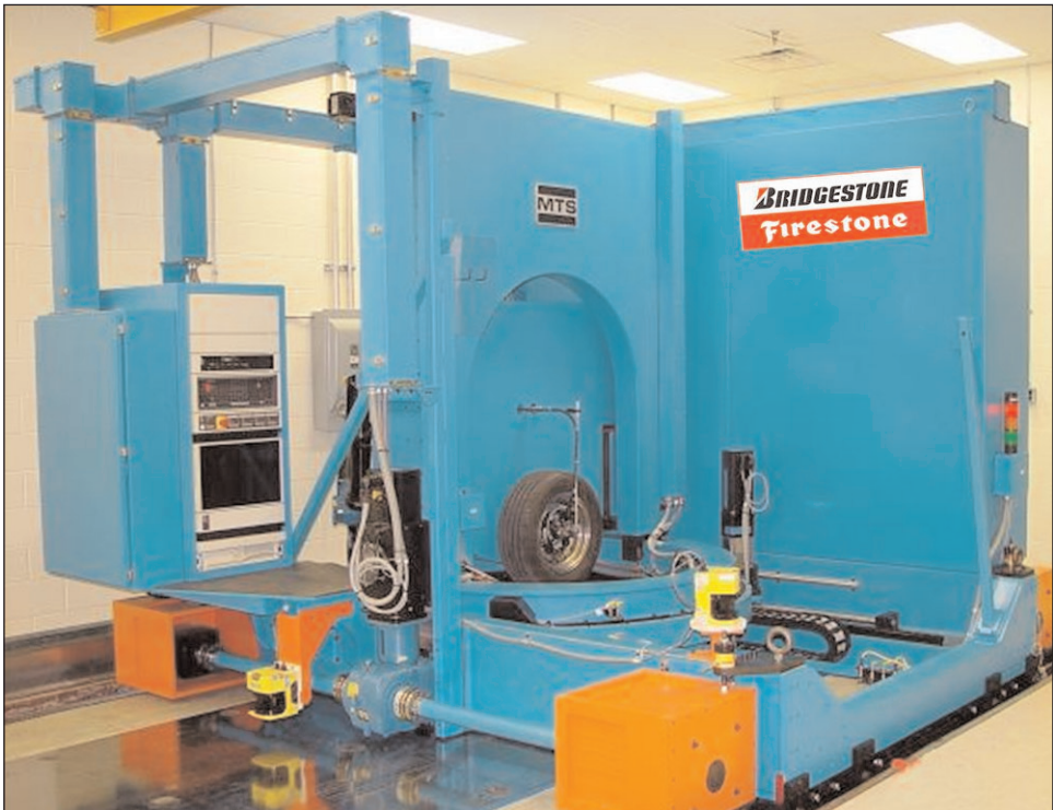
Figure 7.15: A modern, moving carriage, stationary bed, flat-surface machine manufactured by MTS Systems, Inc Bridgestone/Firestone Co.
