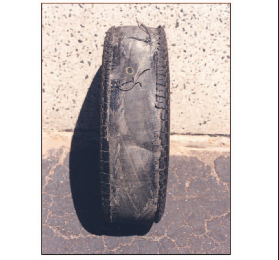
Figure 15.16: Exemplar tire after tread/belt detachment
