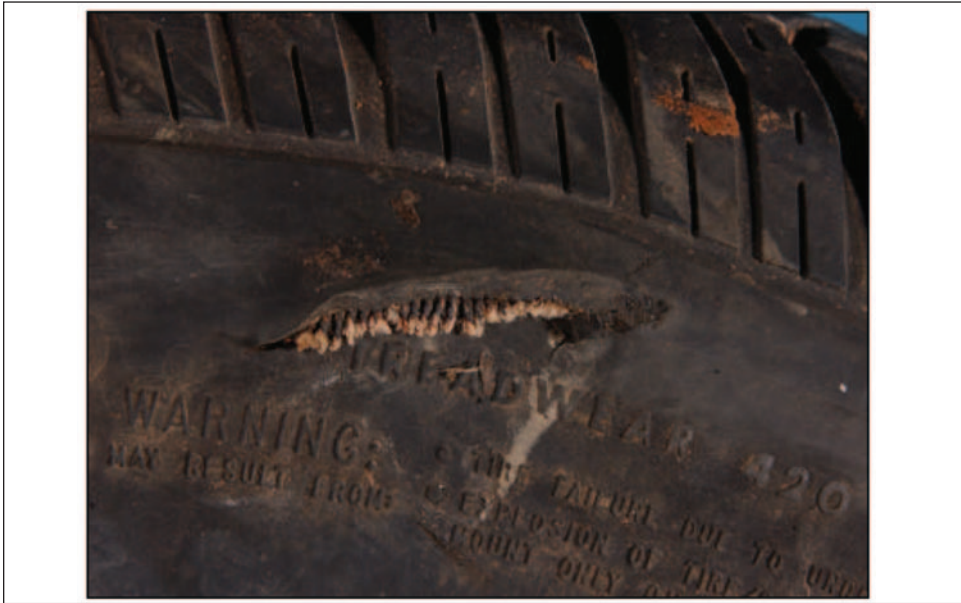
Figure 15.17: Upper sidewall break through to cavity
