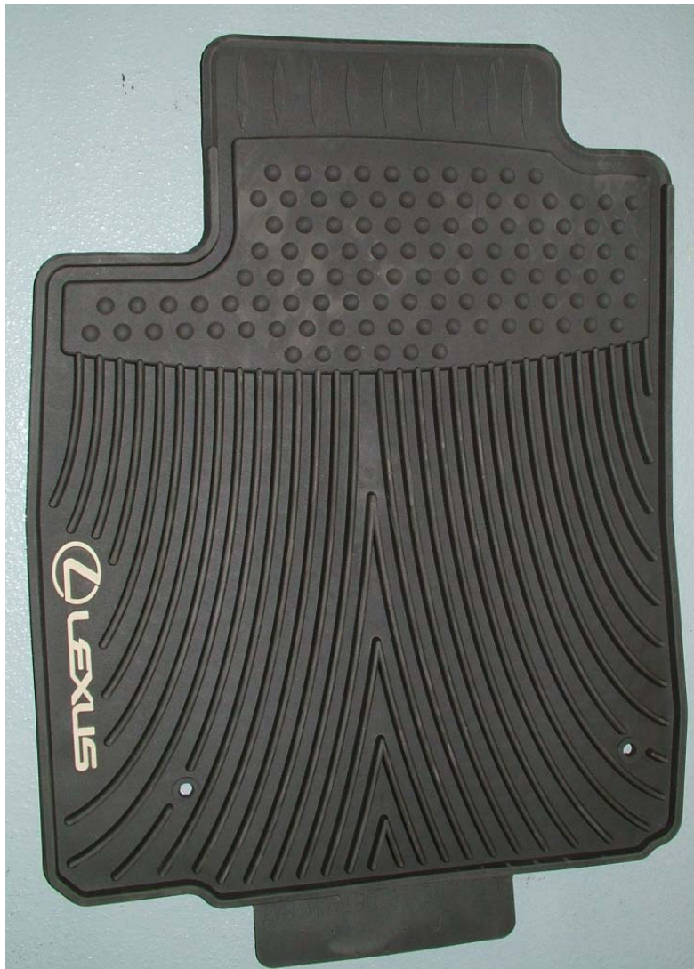
Figure 2 – Lexus All-weather Floor Mat with Retaining Hook Holes at the Bottom
